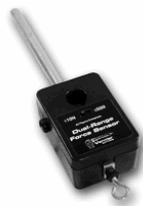
The Dual-Range Force Sensor is a general-purpose device for measuring pushing and pulling forces. It can be used as a replacement for a hand-held spring scale or mounted on a ring stand. It can also be mounted on a dynamics cart to study collisions. Forces as small as 0.01 newtons and as large as 50 newtons can be measured. The Dual-Range Force Sensor can be used for a variety of experiments, including
